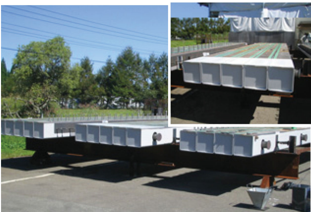
Fig. 10 Panel members composed of steel square tubes
