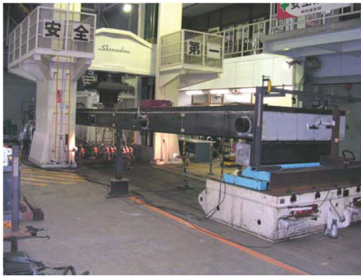
Fig. 3 Loading test condition
