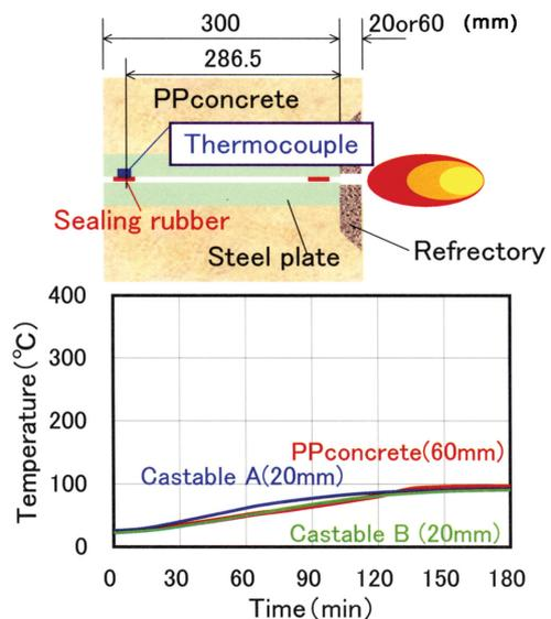
Fig. 6 Temperature of sealing rubber
