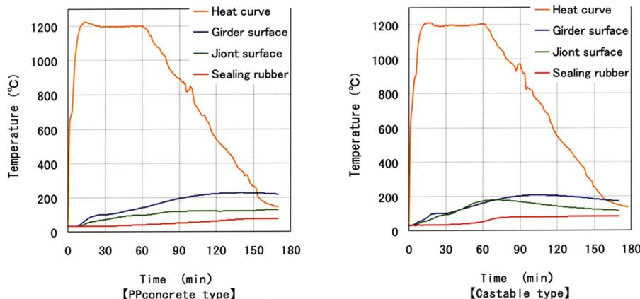
Fig. 10 Time-temperature curve of PP concrete type and castable type
