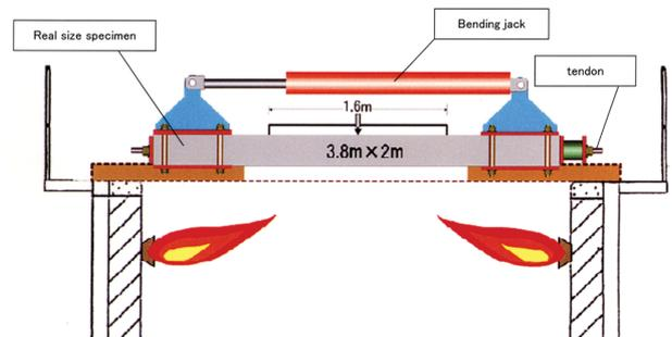
**Fig. 9 Fire test with loading jack**
