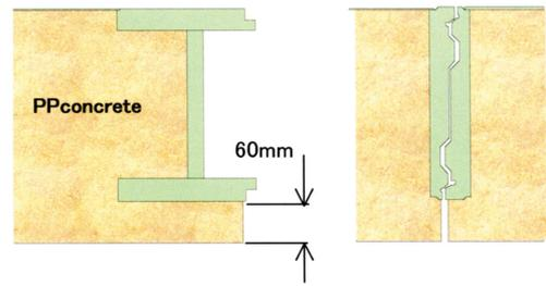
**Fig. 7 Section of PP concrete refractory**
