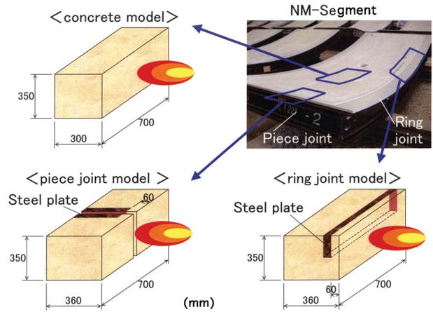
Fig. 2 Specimens of reduction model
