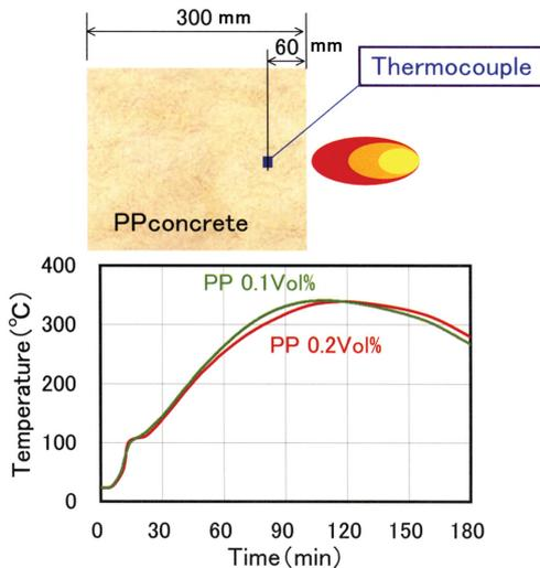
Fig. 4 Temperature of concrete at 60 mm depth
