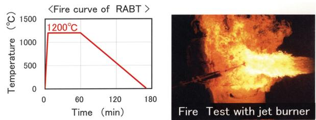
Fig. 3 Fire test for reduction models
