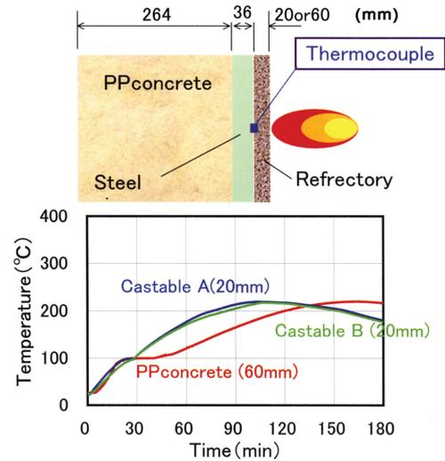
Fig. 5 Temperature of steel surface
