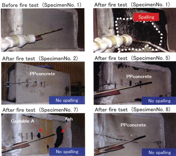
Photo 4 Test results of before and after fire test
