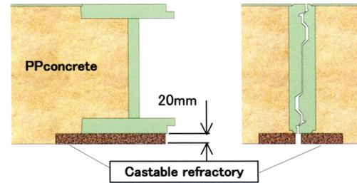
**Fig. 8 Section of castable refractory**
