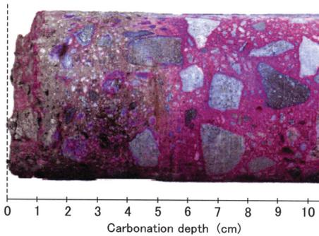
Photo 8 Carbonation after fire test
