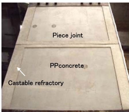
**Photo 6 Specimen of castable refractory**
