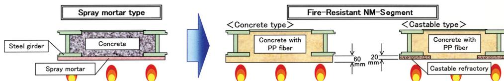
Fig. 1 Structures of Fire-Resistant NM-Segment
