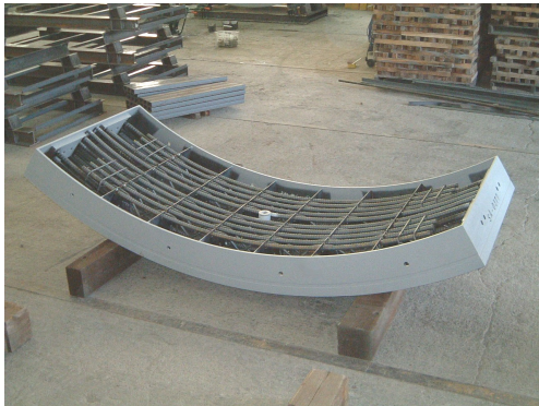
Photo 2 Composite CP segment without concrete
