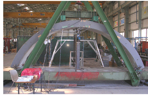
Photo 1 Bending test for joint
