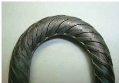
Photo 3 Result of bending test for HDC800/D8
