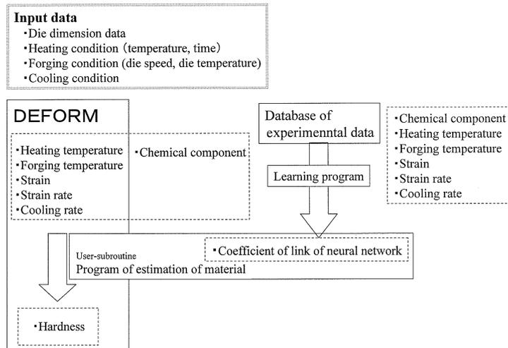
Fig. 5 Estimation system of material distribution of forged part
