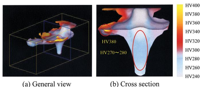
Fig. 7 Hardness distribution of forged part
