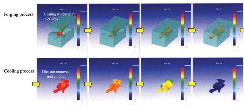
Fig. 6 Temperature distribution of forging and cooling process
