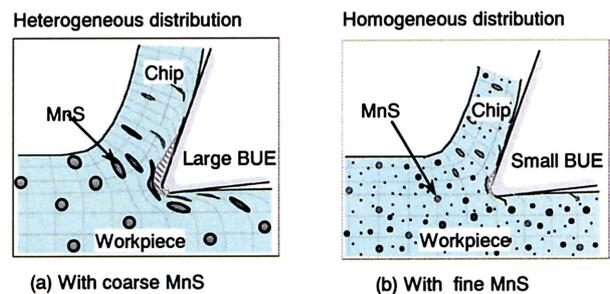
Fig. 2 Schematic view about effect of MnS on BUE formation
