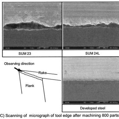
Fig. 5 Effect of number of machined parts on surface roughness and flank wear
