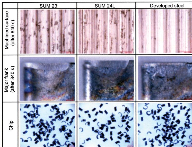
Fig. 9 Optical micrograph of machined surface, tool wear, and chip
