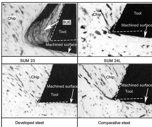
Fig. 4 Cross sectional view of chip formation by QST sample
