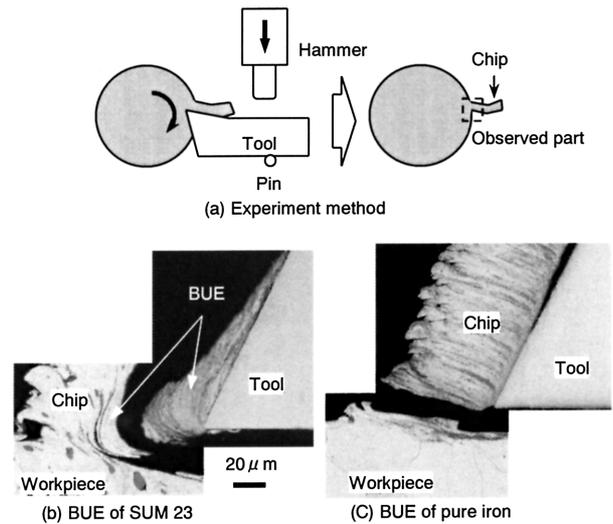
Fig. 1 Cross sectional view of chip formation part by QST
