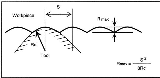
Fig. 8 Surface roughness calculated on geometry
