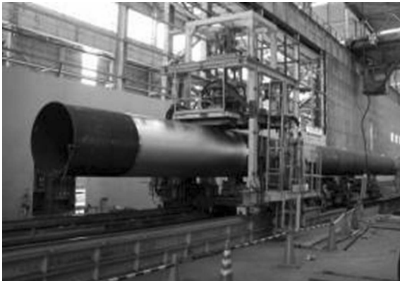
Fig. 5 Appearance of the indirect seam welding equipment
