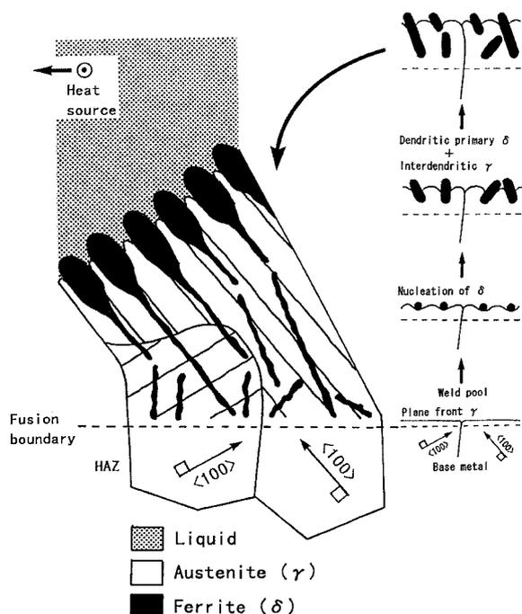
Fig. 4 Schematic illustration on the formation and the growth of ferrite and austenite near the fusion boundary of weld metal solidified in FA mode
