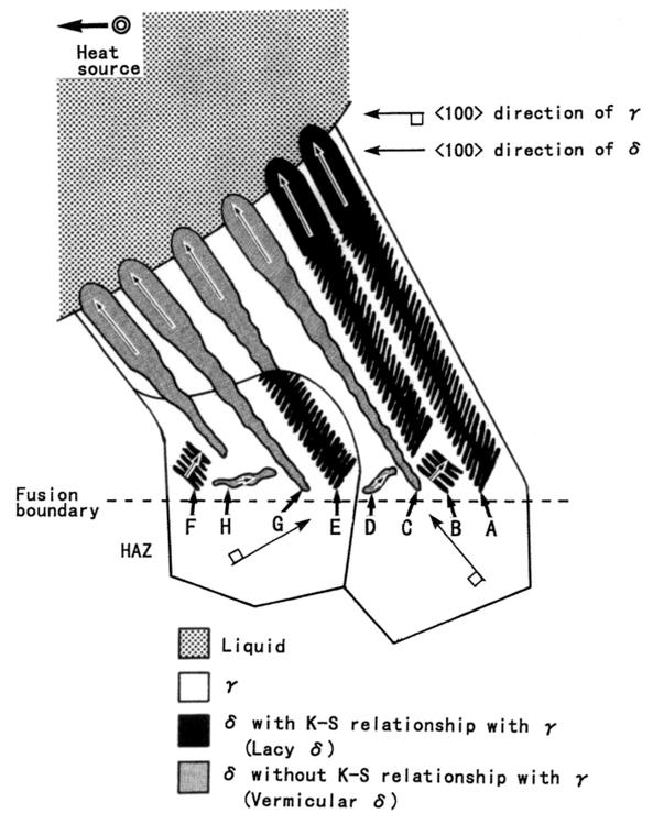
Fig. 7 Schematic illustration of formation process and mechanism for different ferrite morphologies in weld metals solidified in FA mode. (A-H correspond to cases in Fig. 6)
