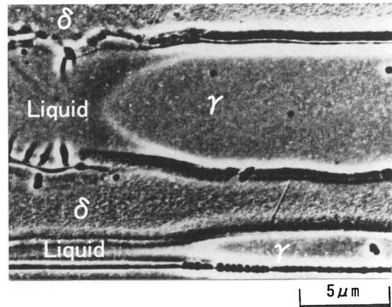
Fig. 3 Growth front of the interdendritic austenite during primary ferrite solidification
