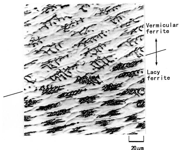
Fig. 1 Typical microstructure as solidified metal of austenitic stainless steel which solidified in FA mode
