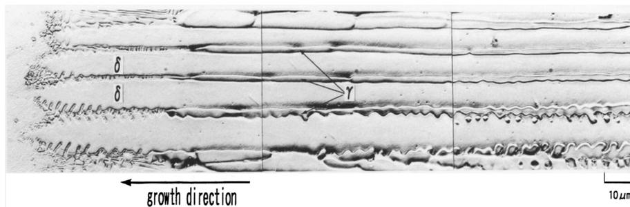
Fig. 2 Microstructural change during solidification in the weld metal obtained by liquid tin quenching method
