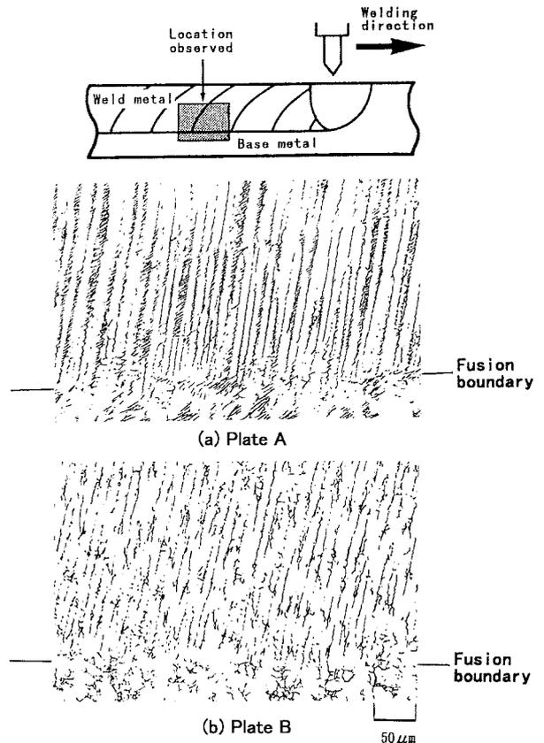
Fig. 9 Microstructures taken near bottom of weld center, parallel to welding direction, in autogenous TIG welds on (a) plate A and (b) plate B in Fig. 8
