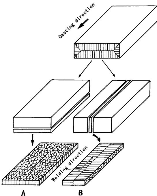
Fig. 8 Schematic illustration of plate preparation from ingot, cutting austenite columnar structure vertically (A) and cutting parallel to austenite columnar structure (B)
