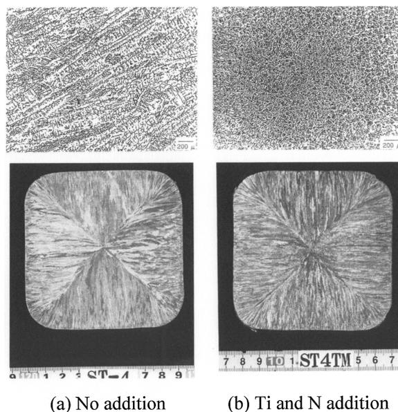
Fig. 5 Microstructures and macrostructures of austenitic stainless steel ingots, (a) no addition, (b) Ti and N addition
