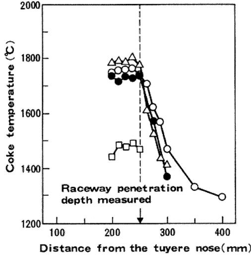
Fig. 5 Coke temperature measured in the raceway and deadman (injection of 0% pre-reduced fine ore)
