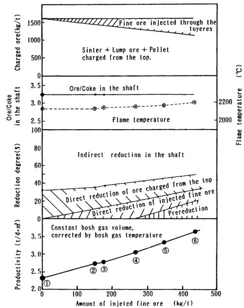
Fig. 2 Example of blast furnace operation injected with fine ore from the tuyere
