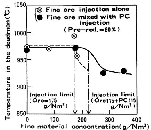
Fig. 7 Relationship between the fine material concentration and the deadman temperature during injection of 60% pre-reduced fine ore alone or mixed with pulverized coal
