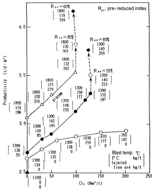
Fig. 3 Productivity in the operation injected a maximum amount of fine ore mixed with pulverized coal
