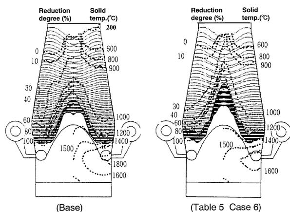
Fig. 8 Simulation results of reduction behavior in the future blast furnace
