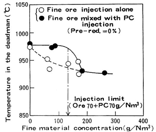
Fig. 6 Relationship between the fine material concentration and the deadman temperature during injection of 0% pre-reduced fine ore alone or mixed with pulverized coal
