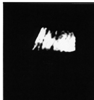
Fig. 2 2D images of raw coal and with swelling pyridine-d5 obtained by spin echo method
