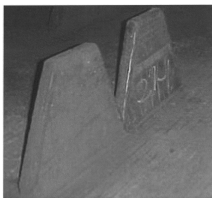
Fig. 4 An appearance of stands attached to a pallet in Kimitsu No. 3 sintering machine
