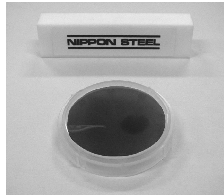
Fig. 1 2-inch silicon carbide epitaxial wafer
