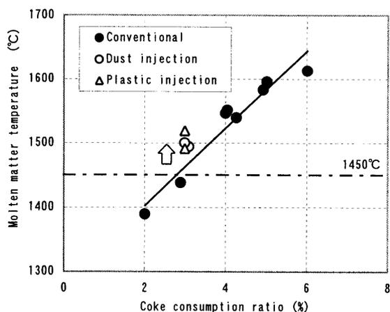
Fig. 4 Effect of coke consumption ratio on molten matter temperature
