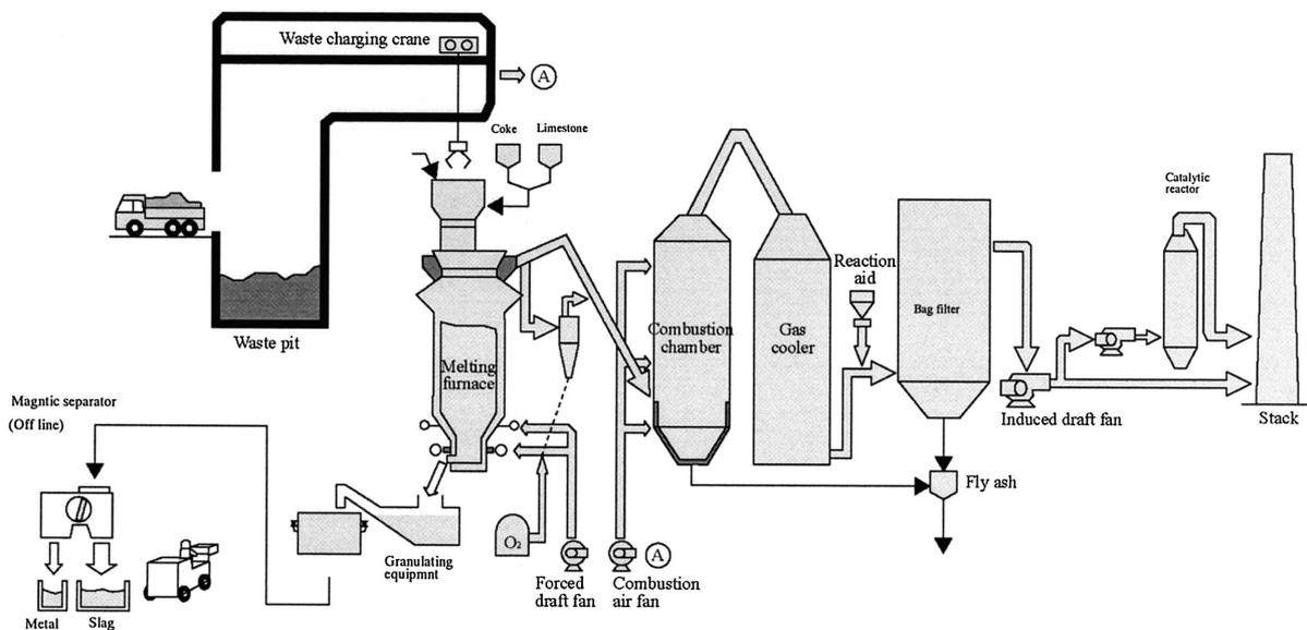
Fig. 2 Flow diagram of direct melting experimental plant
