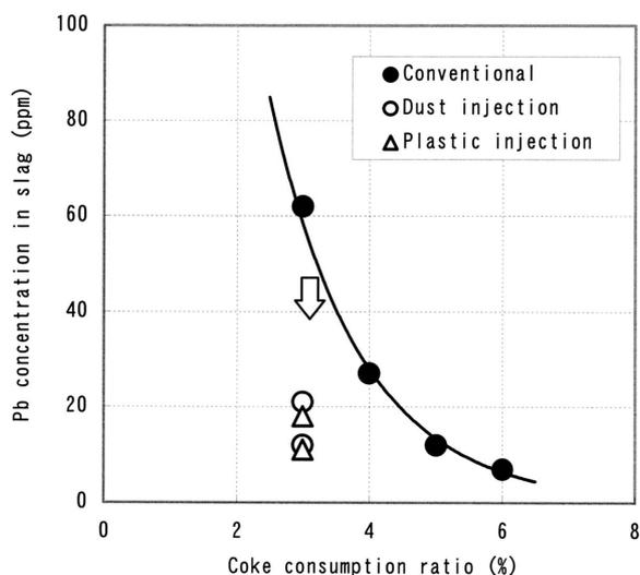
Fig. 5 Effect of coke consumption ratio on Pb concentration in slag
