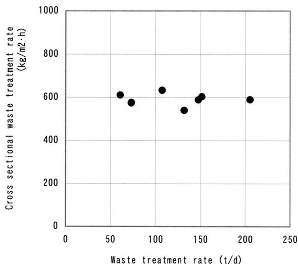
Fig. 11 Cross sectional waste treatment rate in the shaft
