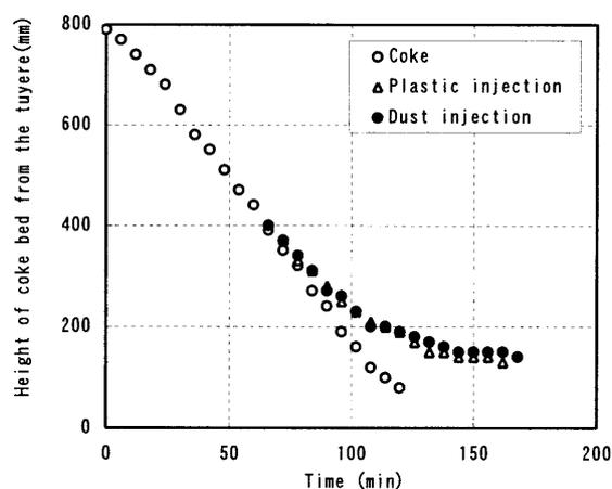
Fig. 1 Change of coke bed height at combustible injection
