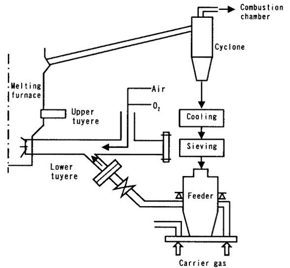
Fig. 3 Flow diagram of combustible dust injection system
