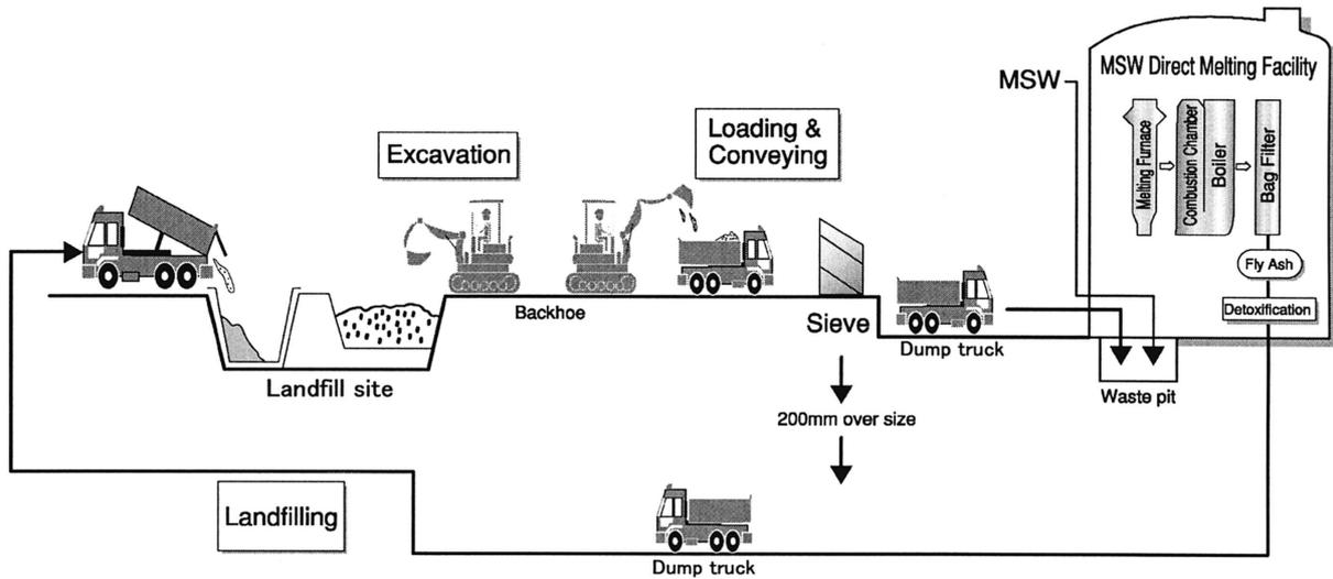
Fig. 9 Flow diagram of treating excavated waste
