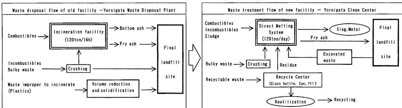
Fig. 8 Waste disposing process flow comparing old and new facilities
