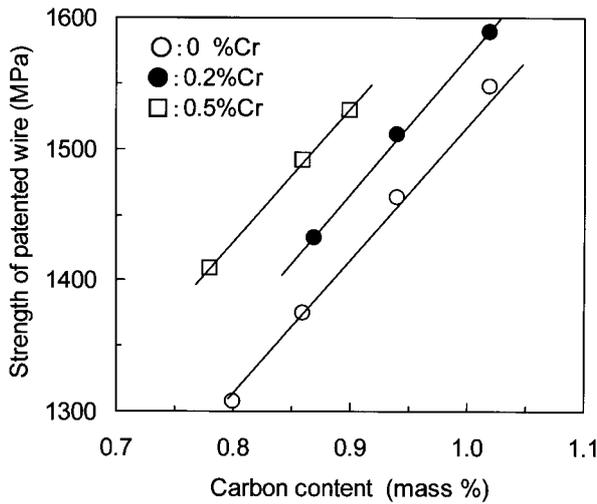
Fig. 1 Effect of C and Cr content on patented wire strength
