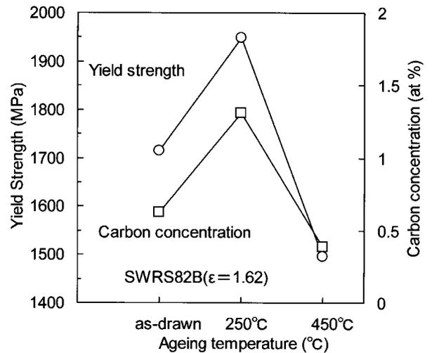
Fig. 10 Variations of yield strength and C concentration in ferrite with aging temperature
