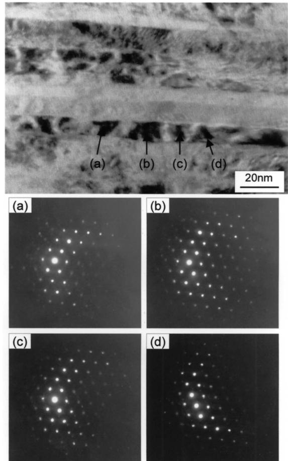
Fig. 6 TEM micrograph and selected area electron diffraction patterns of high carbon steel wire ( $\epsilon = 4.2$ )
