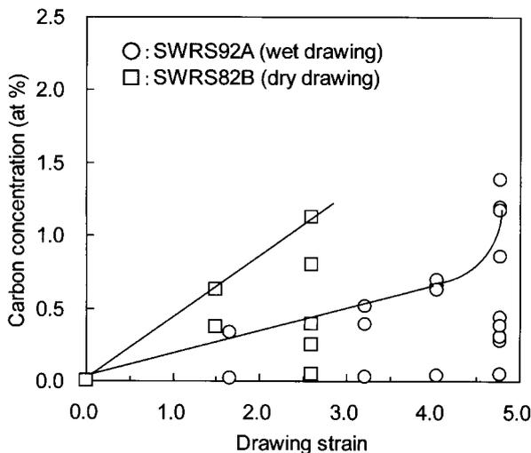
Fig. 8 Variation of carbon concentration in ferrite with drawing strain
