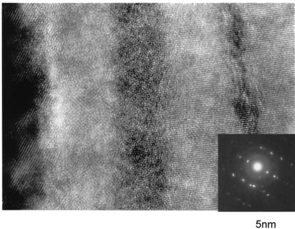
Fig. 5 Lattice image of high carbon steel wire ( $\epsilon = 4.2$ )
