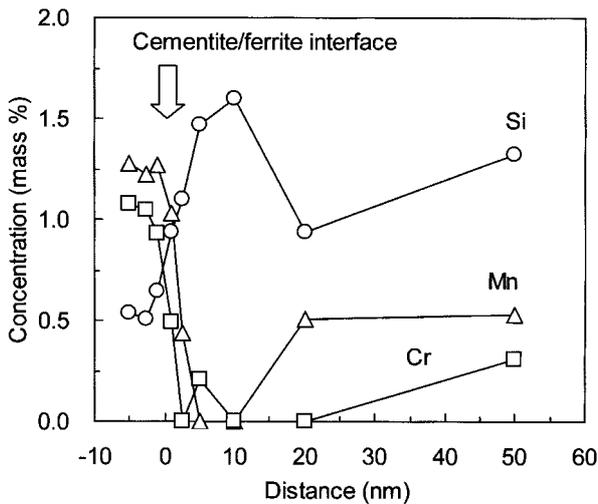
Fig. 4 Distribution of alloying elements across ferrite-cementite interface
