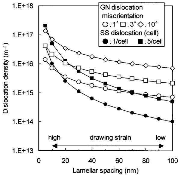
Fig. 7 Relationship between lamellar spacing and dislocation density
