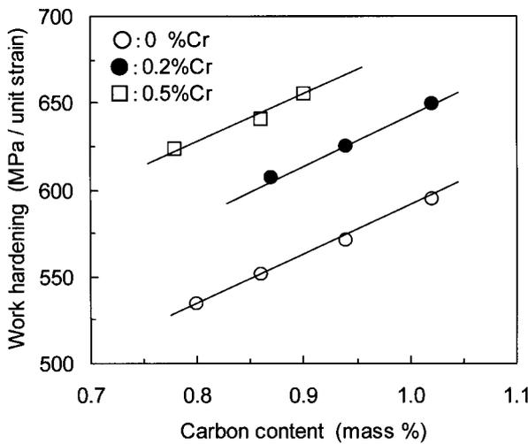
Fig. 2 Effect of C and Cr content on amount of work hardening
