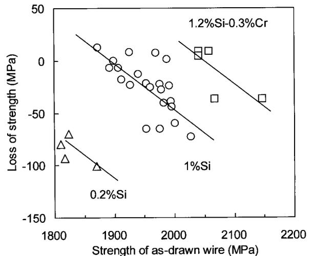
Fig. 3 Effects of as-drawn wire strength and alloying elements on loss of strength during galvanizing
