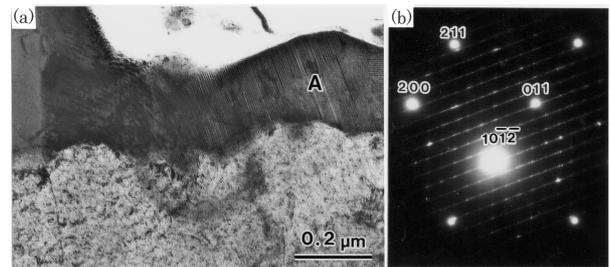
Photo 5 Transmission electron micrograph showing (a) A bright field image of the cross-sectional microstructure around the bottom of a crater, and (b) The selected area diffraction pattern taken from the crystal noted A in the photograph. The diffraction pattern is identified to be the δ-phase.
