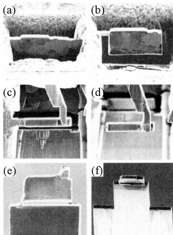
**Photo 3** A series of scanning ion micrographs showing the micro-sampling process
