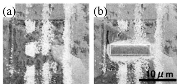
**Photo 2** Scanning ion micrographs indicating the W protective layer deposition process
