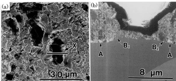
Photo 4 Morphology of craters formed on the galvanized steel observed by a scanning ion microscope (a) The top view of craters, and (b) The cross-section view of the crater noted by line X in photograph (a)
