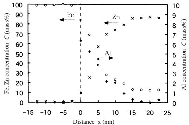
Fig. 2 Change of Fe, Zn and Al concentration along the interface between δ-phase and the steel, measured by EDS analysis. The positive values correspond to the distance from the interface to the galvanizing phase.
