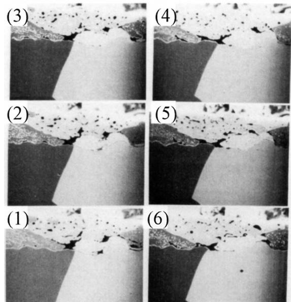
Photo 1 Continuous scanning ion micrographs showing the microstructure of internal oxidation near a steel surface. Cross sections from (1) to (6) are fabricated by a width of  $1\mu\text{m}$ .
