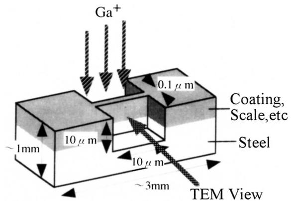
Fig. 1 Schematic diagram of focused ion beam fabrication
