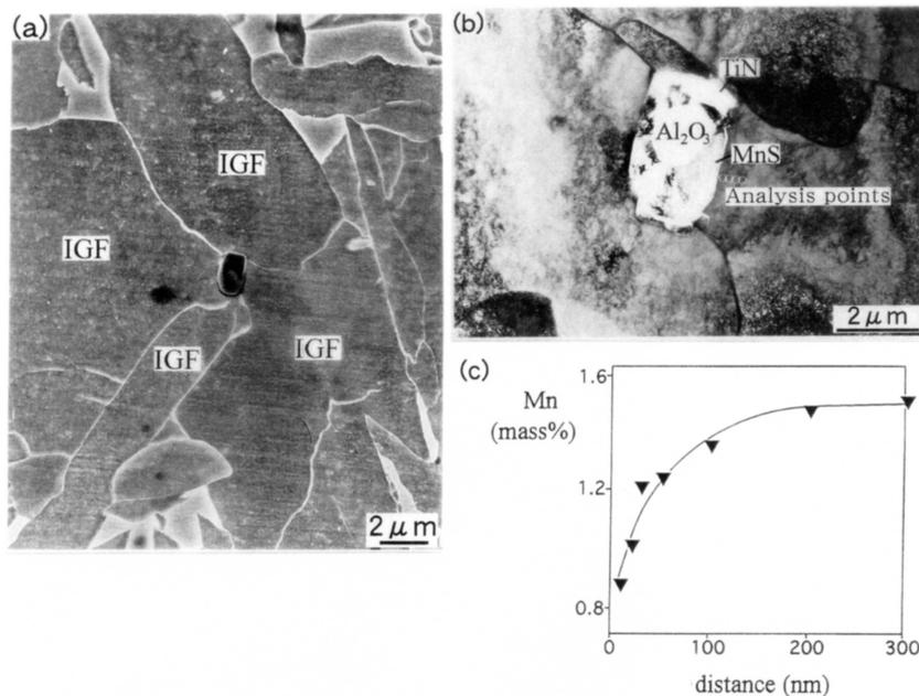
Photo 6 Characterization of the precipitate showing the intra-granular transformation (a) Scanning electron micrograph of the precipitate and intra-granular transformed ferrites, (b) Cross-sectional transmission electron micrograph of the precipitate, and (c) The change in Mn concentration in a region near interface of MnS measured by EDS analysis
