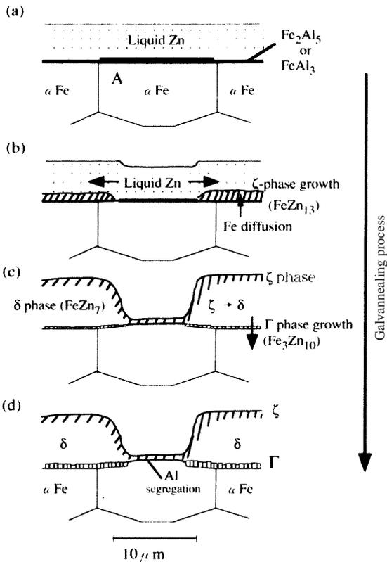
Fig. 3 Schematic diagram indicating the model for the formation of a crater during the galvannealing process
