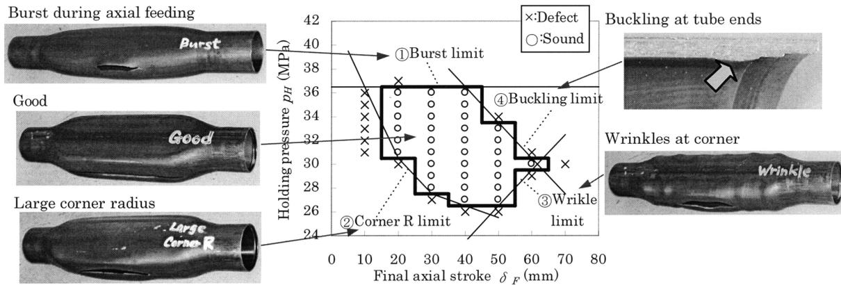
Fig. 6 Forming allowance evaluation for HF
