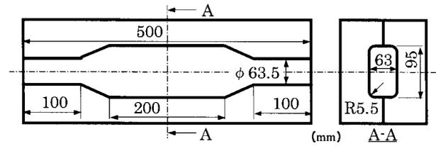
Fig. 2 Die shape for HF tests
