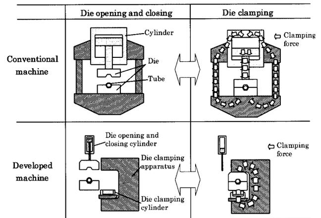
Fig. 10 Comparison of die closing mechanism of HF machine
