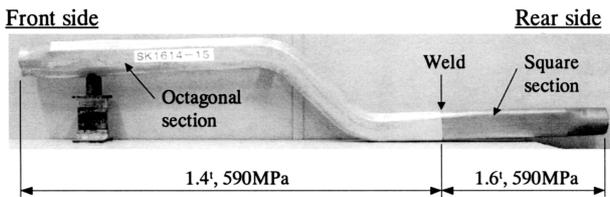
Fig. 12 Forming example by developed HF machine (front side member)
