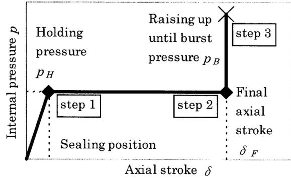
Fig. 3 Loading path in HF tests
