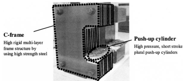
Fig. 11 C frame structure of developed HF machine
