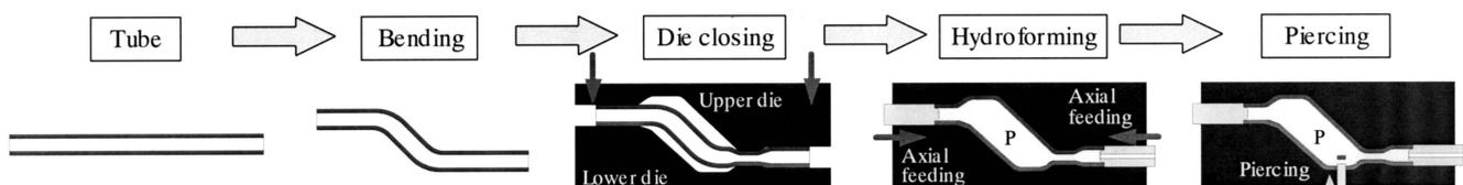
Fig. 1 General hydroforming process
