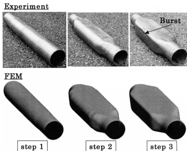
Fig. 4 Deforming shape during HF process
