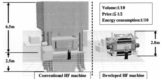
Fig. 9 Comparison of HF machine size (die closing force: 35,000 kN)
