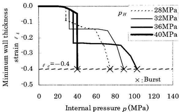
(a) Minimum wall thickness strain during hydroforming
