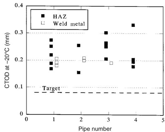
Fig. 9 CTOD test results of the seam weld centerline and heat affected zone
