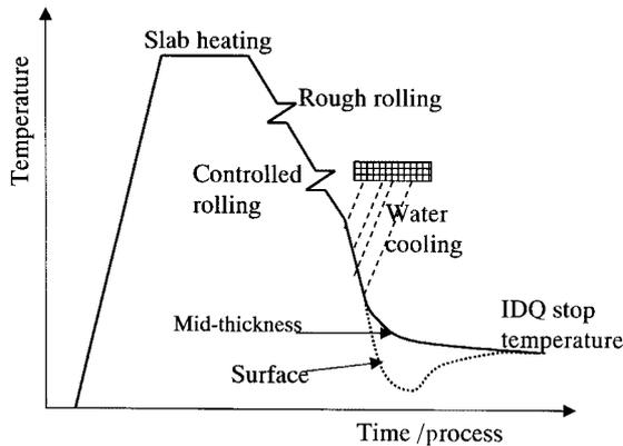
Fig. 2 Schematic illustration of IDQ process
