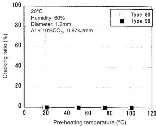
Fig. 6 Cold cracking sensitivity of girth weld - results of y-groove weld cracking test
