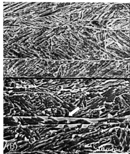
Photo 1 Effect of microstructure on CVN value (microstructure, IDQ stop temperature, CVN value at -40°C) (A) Lower bainite, 453°C, 258J, (B) Upper bainite, 533°C, 167J
