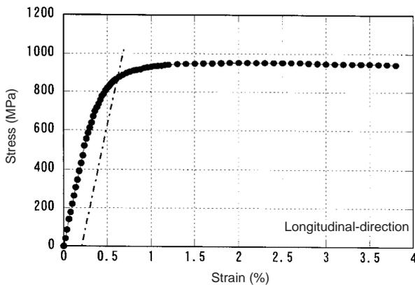
Fig. 8 Typical stress-strain curve in the longitudinal direction
