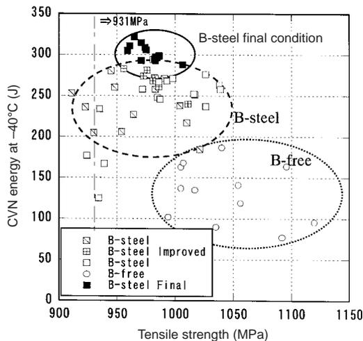
Fig. 3 Effect of alloy system on the balance of tensile and CVN value
