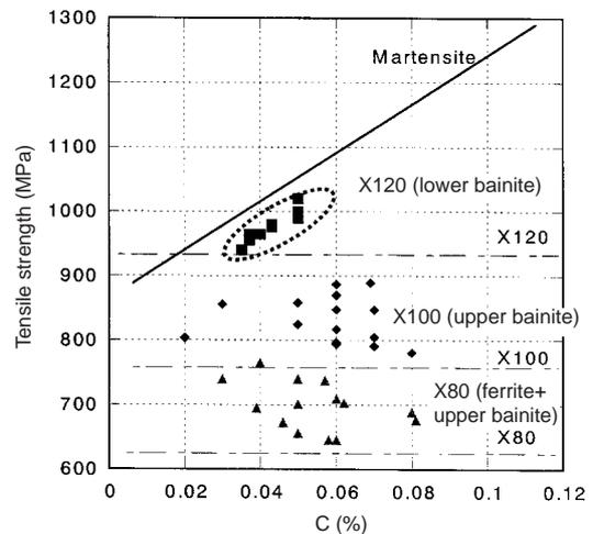
Fig. 5 Relationship between C content and tensile strength for high strength linepipe
