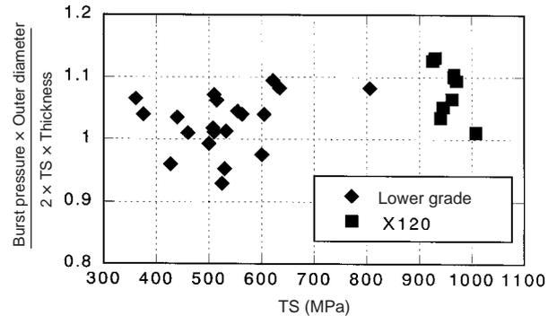
Fig. 10 Burst pressure as a function of tensile strength
