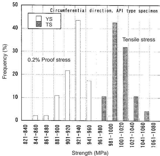
**Fig. 11** Distribution of YS and TS for pipes manufactured in a small scale commercial production
