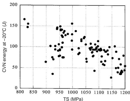
Fig. 7 Relationship between tensile strength and CVN value of submerged arc weldmetal
