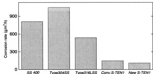
Fig. 3 Immersion test results under 50% H<sub>2</sub>SO<sub>4</sub> at 70°C
