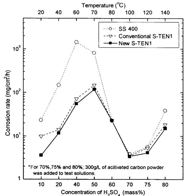
Fig. 2 Immersion test results under the SO<sub>3</sub>-10% H<sub>2</sub>O equilibrium state of sulfuric acid
