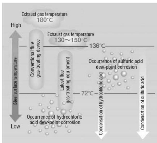
Fig. 1 Schematic diagram of acid dew corrosion mechanisms (flue gas: SO<sub>3</sub>: 6ppm, HCl: 300ppm, H<sub>2</sub>O: 30%)
