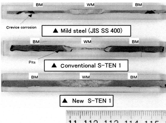
**Photo 6** Cross-section of welded joints after 4 months immersion test in HCl pickling pot
