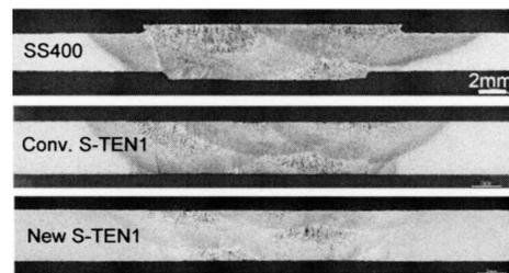
Photo 4 Cross-section of welded joints after 20% H<sub>2</sub>SO<sub>4</sub> immersion
