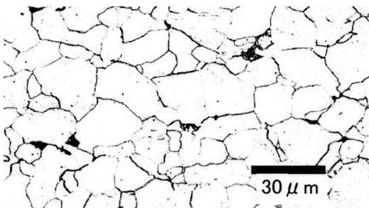
Photo 2 Typical microstructure of new S-TEN™1
