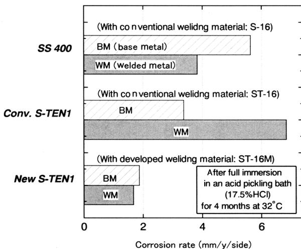
**Fig. 7** Corrosion loss in thickness of welded joints in acid pickling bath
