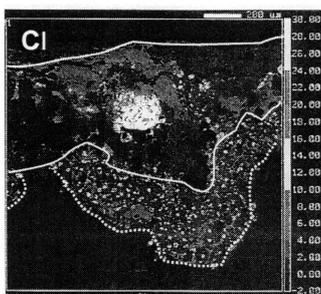
**Photo 1** SE-image of the corroded inner cylinder and distribution of chlorides
