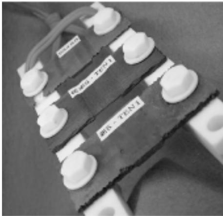
**Photo 5** Appearance of welded joints after 4 months immersion test in HCl pickling pot
