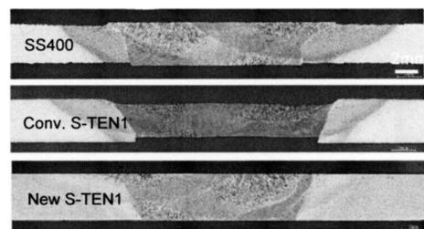
Photo 3 Cross-section of welded joints after HCl immersion tests
