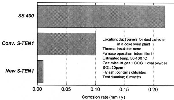
Fig. 6 Corrosion loss in thickness of duct panels at coke oven gas, where sulfuric acid dew corrosion involving chloride-containing ashes
