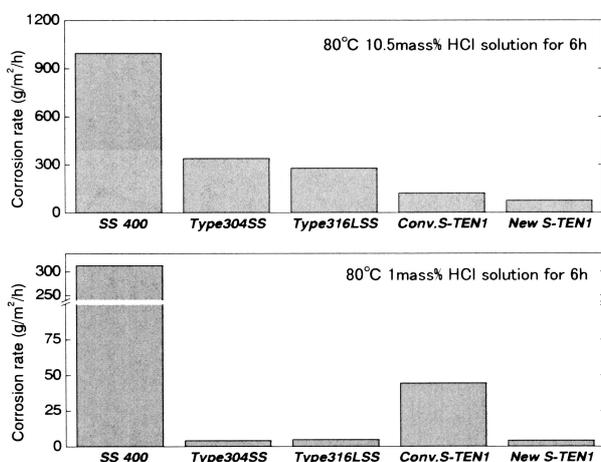
**Fig. 4 Immersion test results under HCl solutions at 80°C**
