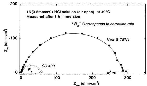
**Fig. 8** Cole-Cole plots of new S-TEN<sup>TM</sup>1 in 1N HCl solution by EIS
