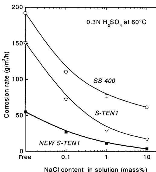
**Fig. 5 Effect of chlorides on corrosion rate of new S-TEN<sup>TM</sup>1 in dilute H<sub>2</sub>SO<sub>4</sub> solution**
