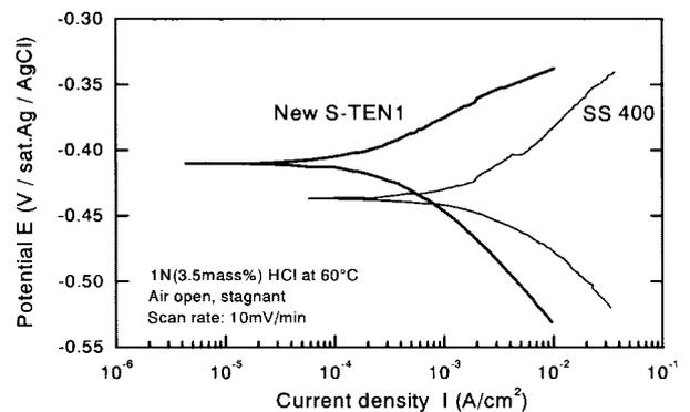
**Fig. 9** Polarization curves of new S-TEN<sup>TM</sup>1 in HCl solution
