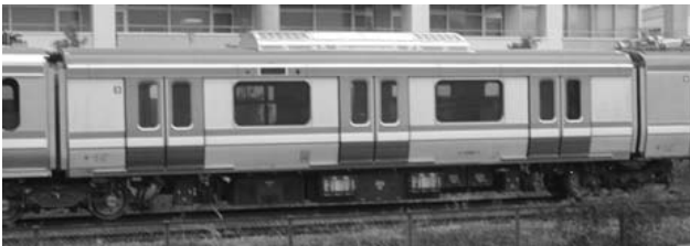
Fig. 3 Prototype cars of AC train constructed using developed honeycomb panels
