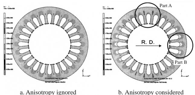
**Fig.4** Distribution of iron loss when anisotropy is considered
