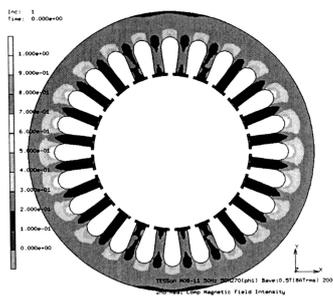
Fig.6 Calculated result of iron loss distribution
