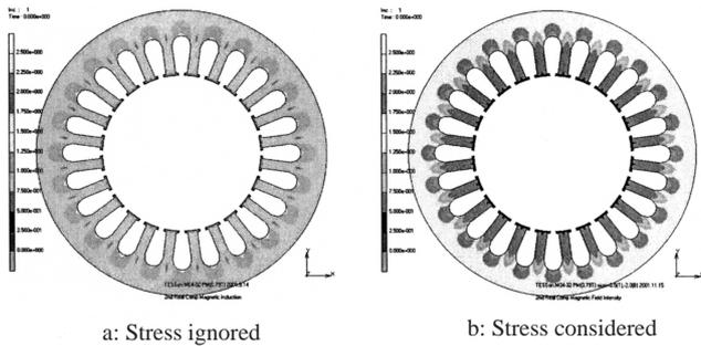
Fig.5 Distribution of iron loss when stress is considered
