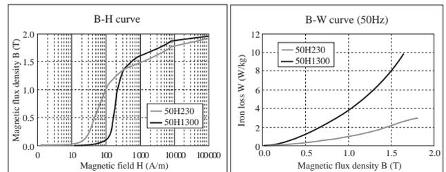
**Fig.2** Magnetic properties of 50H230 and 50H1300
