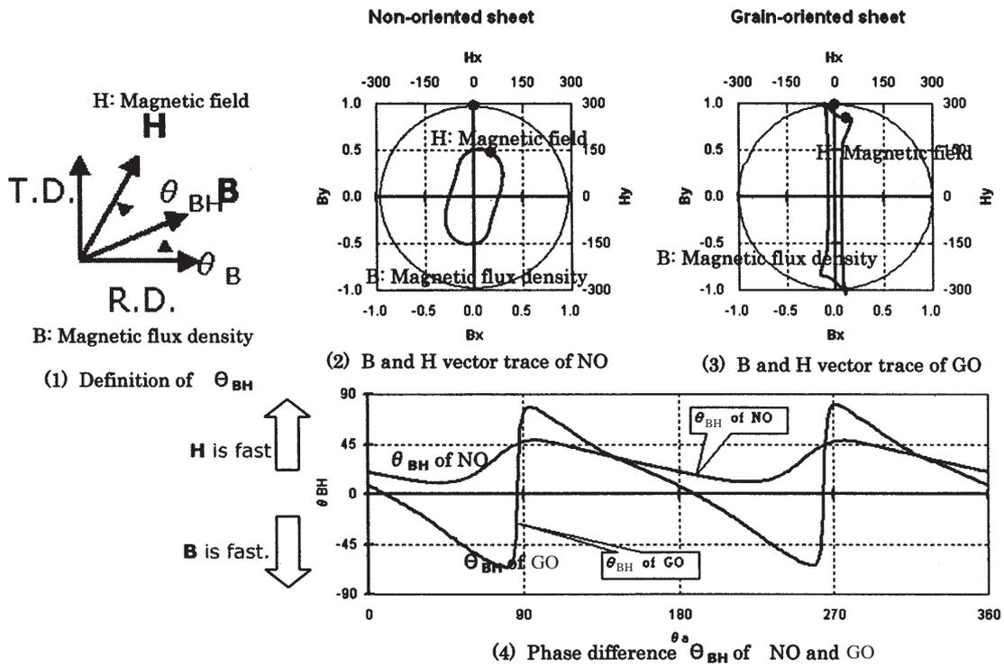
Fig.7 Basic measured results by 2-dimensional vector magnetic measurement method
