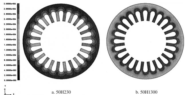
**Fig.3** Distribution of iron loss of 50H230 and 50H1300
