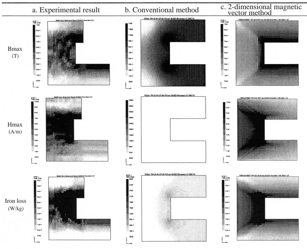
Fig.8 Comparison of magnetic properties, among the measured result, calculated result by the conventional method and calculated result by 2-dimensional magnetic vector method
