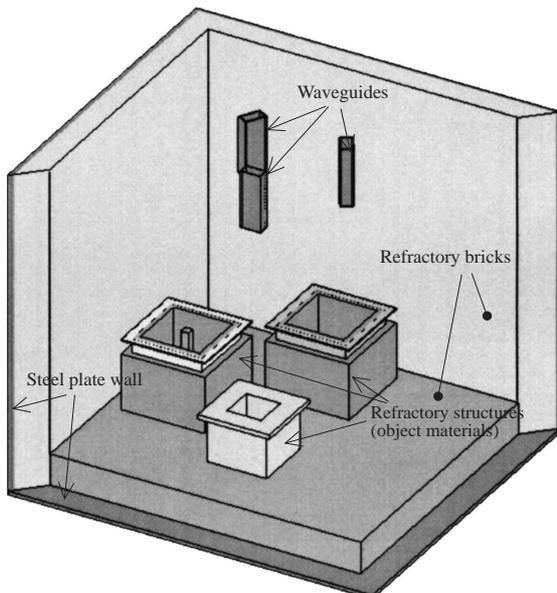
**Fig. 2** Drying chamber model surrounded by steel plates and refractory bricks
