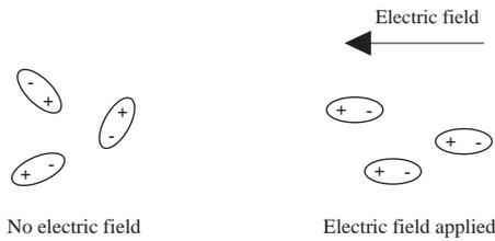
Fig. 1 Oriented polarization of molecules and microwave electric field
