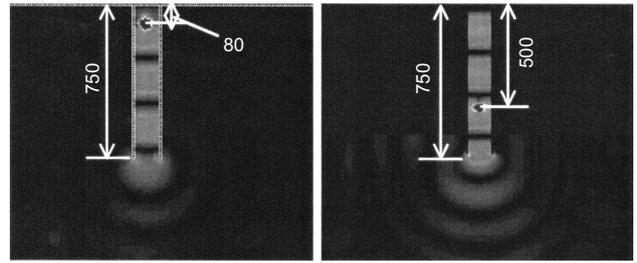
**Fig. 3** Influence of point source position in waveguide (electric field intensity)
