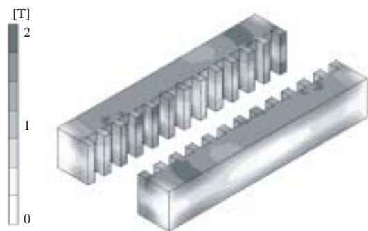
Fig. 5 Analysis example of iron core magnetic flux density distribution
