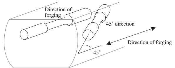
**Fig. 2 How to cut out test pieces from the raw material**
