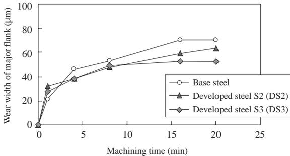
**Fig. 11** Relationship between cutting time and the wear width of major flank when turning the peripheral
