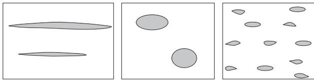
(a) Normal (b) Spheroidized (c) Finely dispersed
