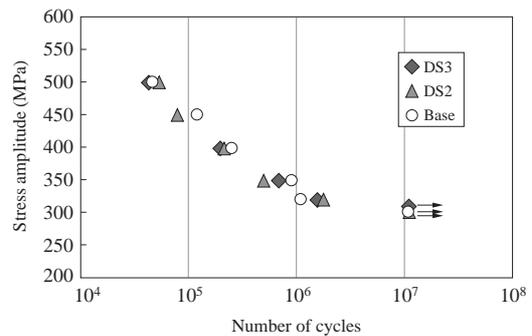
**Fig. 14** Fatigue property of test pieces at 45° to forging direction
