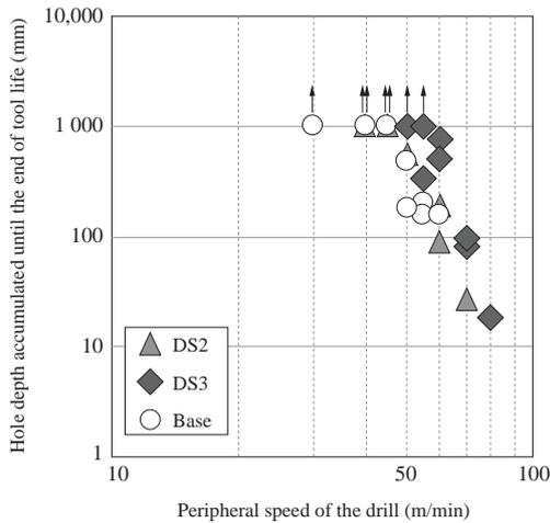
**Fig. 5 Relationship between peripheral speed and accumulated hole depth**
