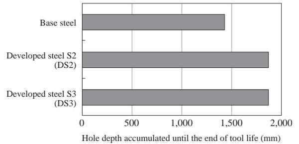
**Fig. 8 Results of evaluation of drill life in deep hole drilling**
