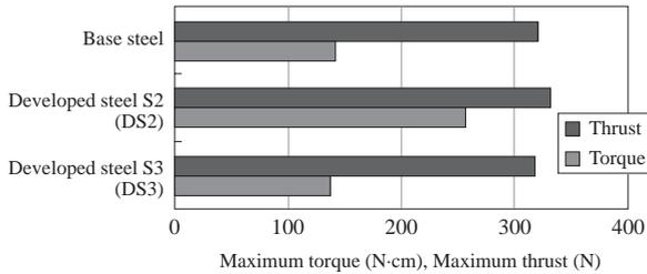
**Fig. 10** Cutting forces when drilling a deep hole
