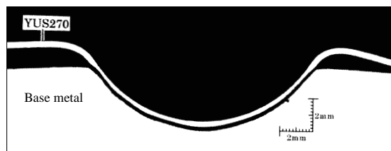
Photo 3 Sectional micrograph of test pieces after impact test (YUS270: 0.4 mm thick)
