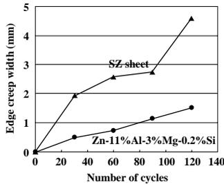
Fig. 7 Edge creep behavior at cyclic corrosion test
