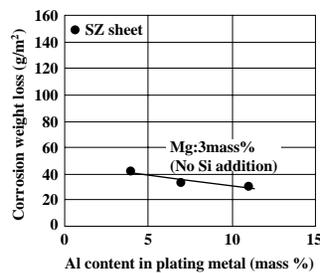
Fig. 2 Influence of Al content in plating metal on corrosion weight loss at 500-h SST
