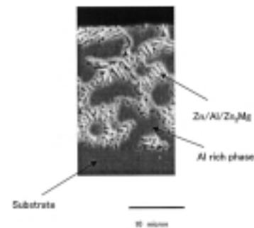
Fig. 6 Sectional micrograph of Zn-11%Al-3%Mg-0.2%Si-plated sheet
