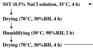
Fig. 1 Condition of cyclic corrosion test
