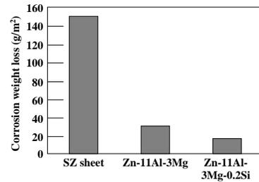
Fig. 4 Influence of Si content in plating metal on corrosion weight loss at 500-h SST
