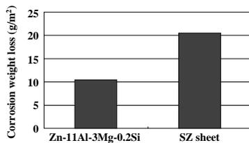
Fig. 9 Corrosion weight loss at 1-year outdoor exposure test in Okinawa
