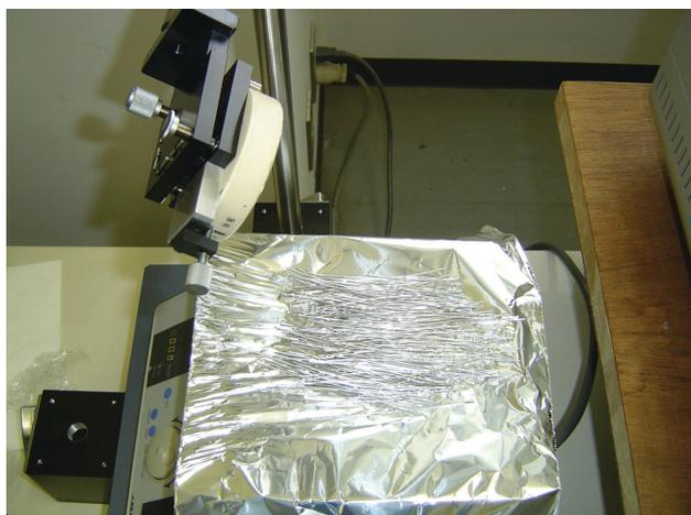
Photo 2 Analysis of wire surface by infrared emission spectrometry
