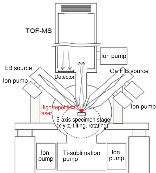
Fig. 1 Schematic diagram of FIB-EB-TOF-SIMS apparatus
