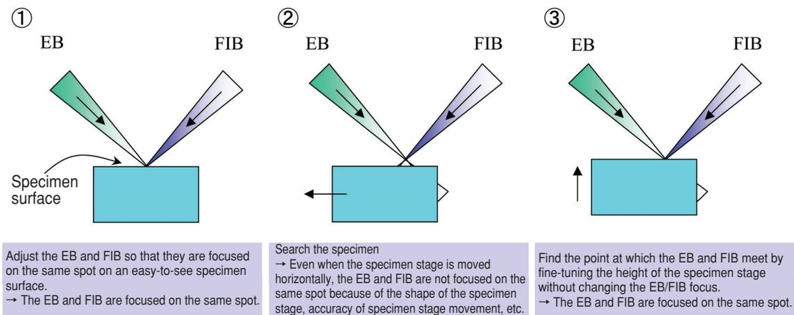
**Fig. 2** Observation procedure of specific area by both electron beam and FIB
