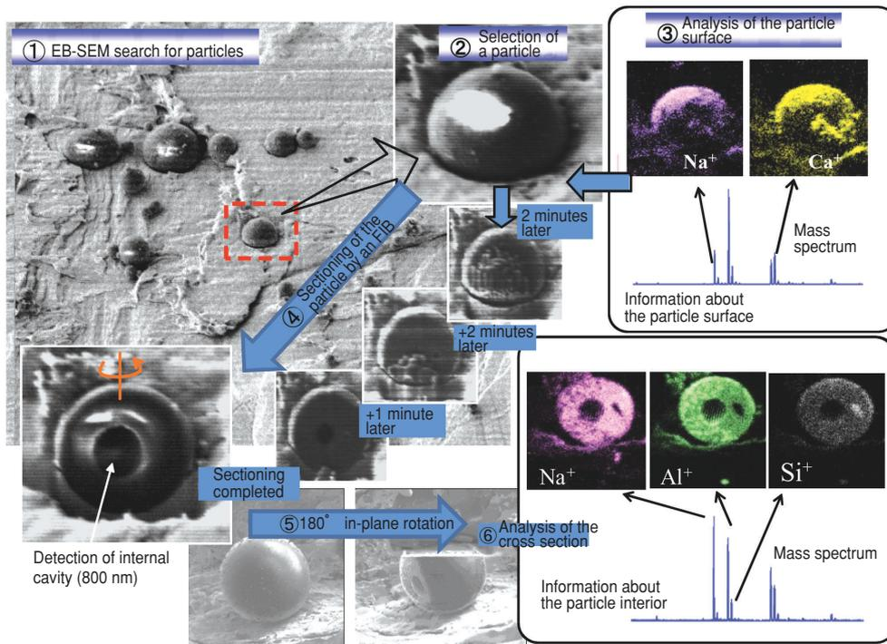
**Fig. 3** Analytical procedure of surface and inner part of a particle
