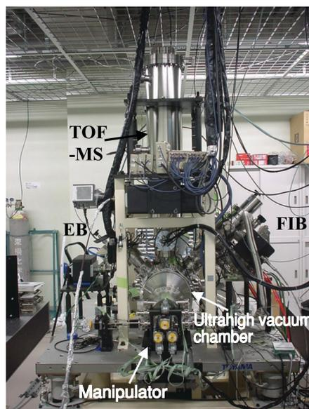
Photo 1 Photograph of FIB-EB-TOF-SIMS apparatus
