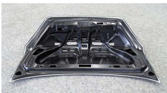
Fig. 9 Trunk lid inner manufactured with high-temperature blow forming A less expensive aluminum alloy developed by Nippon Steel and Furukawa-Sky is employed.
