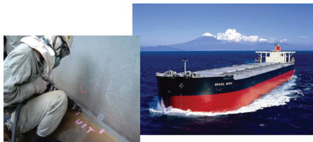
Fig. 8 UIT treatment in ore-carrier; “Brazil Maru” (Photo by Mitsui Engineering & Shipbuilding Co., LTD)
