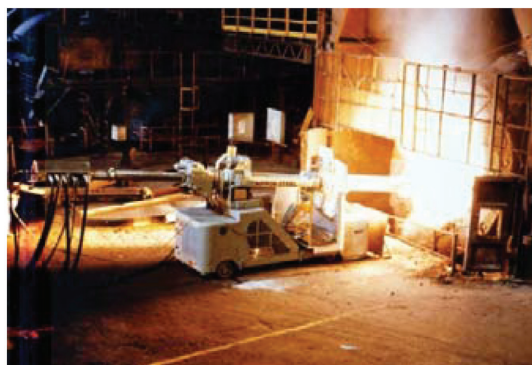
Fig. 7 Flame gunning repairing machine for a BOF
