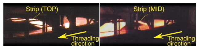
Fig. 17 Examples of unstable strip behavior during threading at a hot strip mill
