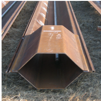
Fig. 8 Hat-shaped steel sheet pile with pile tip enclosure
