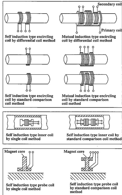
Fig. 6 Classification of eddy current test methods
