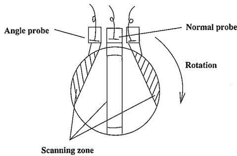
Fig. 8 Principle of ultrasonic test of round bars
