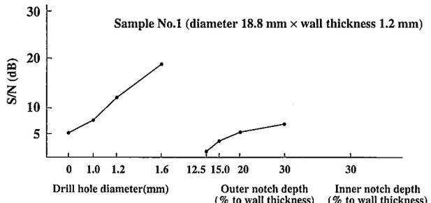
Fig. 7 Detection characteristics of eddy current test (joint test)
