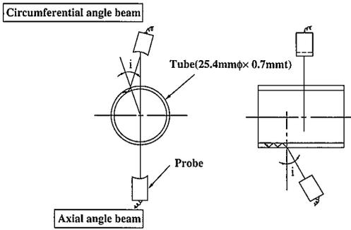
Fig. 3 Ultrasonic test method
