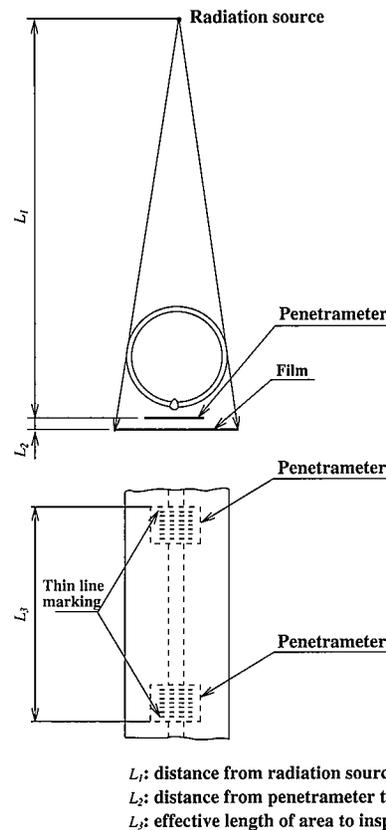
Fig. 2 Arrangement for X-ray radiography of longitudinal welded seam of tube
