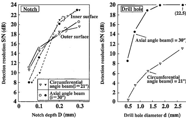
Fig. 5 Detection characteristics of ultrasonic test
