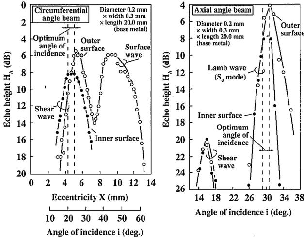
Fig. 4 Relation between angle of incidence and echo height
