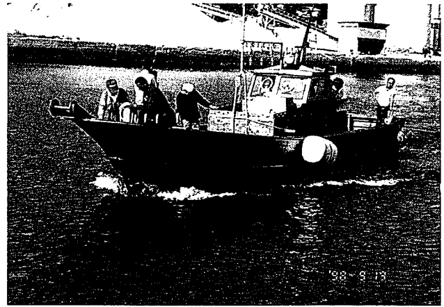
Photo 4 Small ship entirely made of titanium and launched in Karatsu, Saga Prefecture in 1998.
