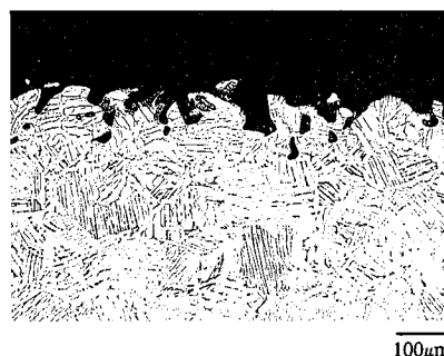
Photo 1 Cross section through surface layer of Ti-6Al-4V alloy HIP compact
