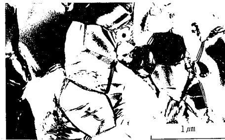
Photo 5 Transmission electron microstructure of 0.2% hydrogenated Ti-6Al-4V alloys after treatment B ( \alpha_M structure formation and 60% hot rolling in \alpha + \beta phase region) and dehydrogenation annealing
