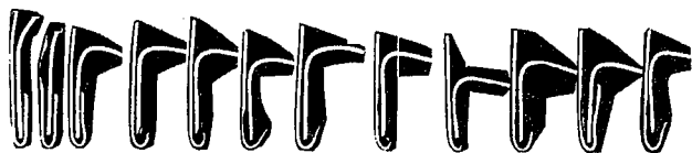
Photo 1 Corrosion of door hem flange of automobile run for 10 years in snow-belt region
