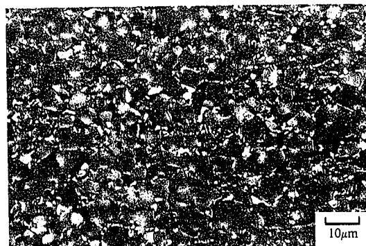
Photo 2 Microstructure of 590-MPa cold rolled retained austenite high-strength steel sheet (blue: ferrite, brown: bainite, white: austenite)
