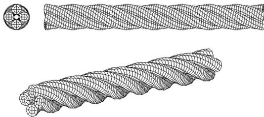
Fig. 3  $1 \times 4 \times 0.11$  strand model for FEM
