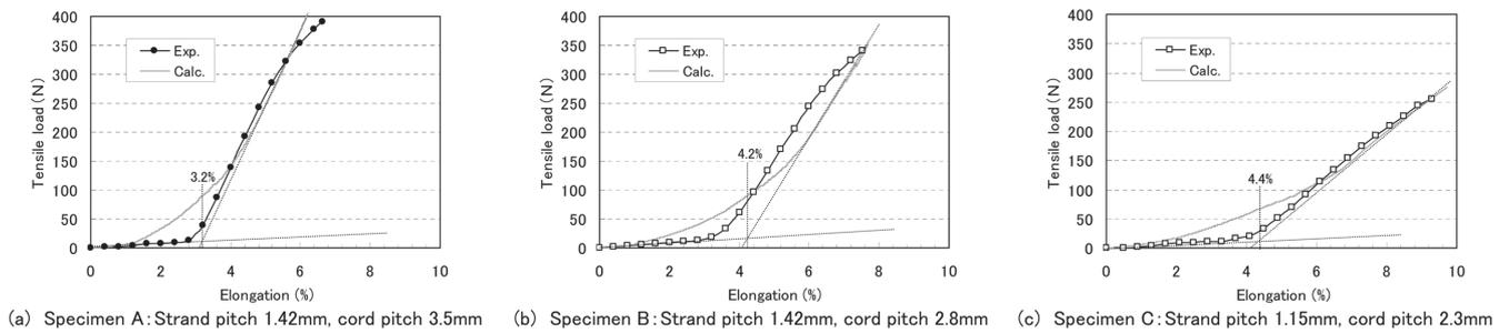
Fig. 10 Comparison with the experimental results and the calculated results, load-elongation curve of  $5 \times 4 \times 0.11$  cord
