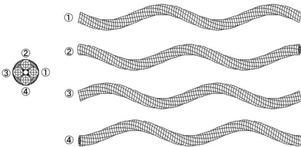
Fig. 6 Simple springs model which decomposed  $1 \times 4 \times 0.11$  strand
