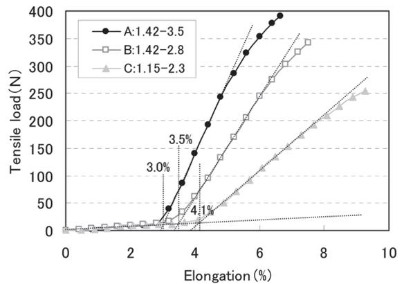
Fig. 8 Load-elongation curves of  $5 \times 4 \times 0.11$  cord
