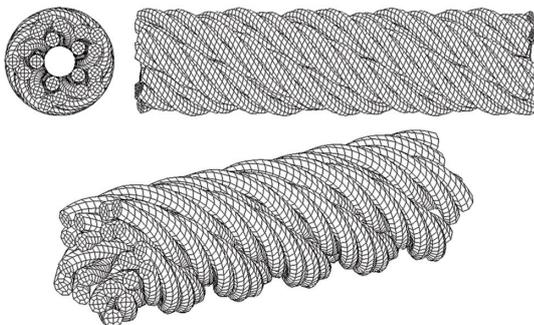
Fig. 4  $5 \times 4 \times 0.11$  cord model for FEM
