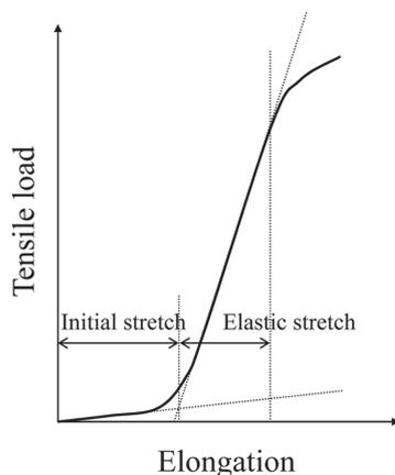
Fig. 1 Model diagram of load-elongation curve of steel cord
