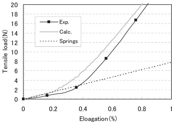
Fig. 7 Load-elongation curves of  $1 \times 4 \times 0.11$  strand
