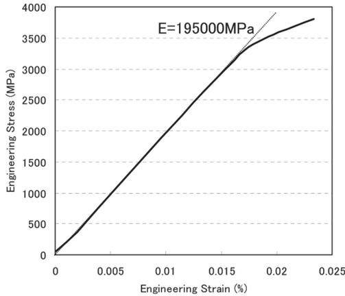
Fig. 2 Stress-strain curve of steel wire
