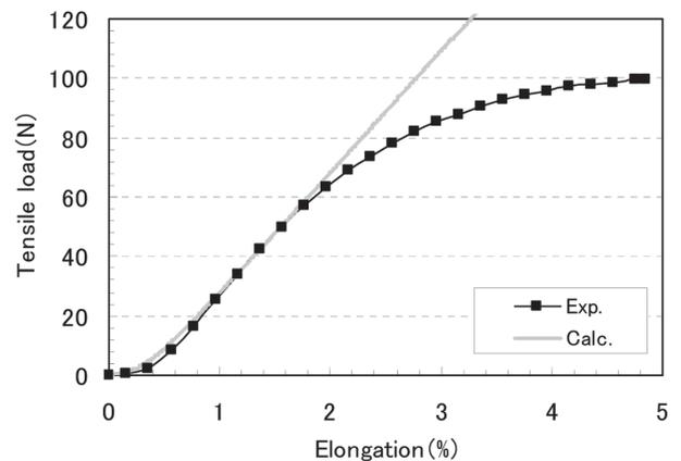
Fig. 5 Load-elongation curve of  $1 \times 4 \times 0.11$  strand
