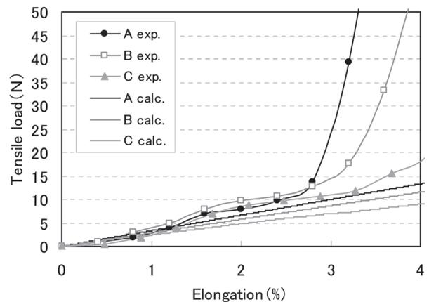
Fig. 9 Comparison with the experimental results and the calculated results by simple springs model
