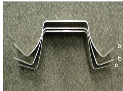
Photo 1 Hat-shaped bending samples a: Aluminum alloy in cold forming b: Aluminum alloy in warm forming at 250°C c: Steel in cold forming
