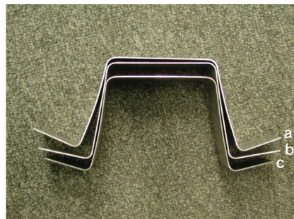
Photo 2 Hat-shaped bending samples a: Aluminum alloy in warm forming at 10kN in BHF b: Aluminum alloy in warm forming at 150kN in BHF c: Steel in cold forming at 10kN in BHF
