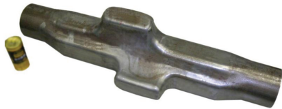
Fig. 5 Forming of two branches in right angles to each other 15)
