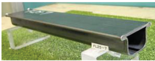
(a) Formed under internal pressure kept by flat seal technology
