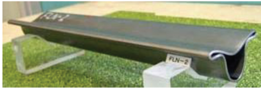
(b) Formed without internal pressure
