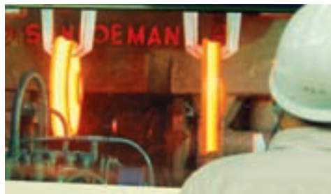
Manufacturing process for railway wheels at the Osaka Steel Works. (Shareholders with more than 10,000 shares are eligible.)
