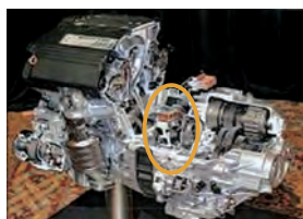
Example of high-efficiency motor using electromagnetic steel sheet
