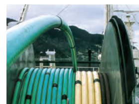
Super 13 Cr steel pipe for seabed pipeline
