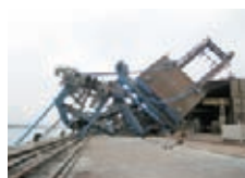
A crane was damaged by a tsunami-wrecked ship.
