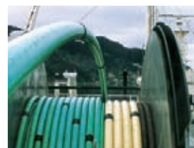
Super 13 Cr steel pipe for seabed pipeline
