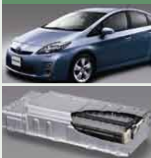
Hybrid vehicle (above) and nickel-hydrogen battery (below) (Toyota Motor Corporation)
