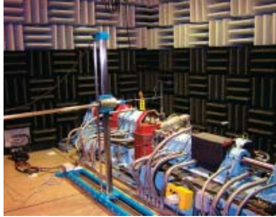
High-speed rotational load test equipment in an anechoic chamber used exclusively for testing train drive units
