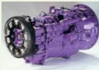
Permanent magnet-type ECB retarder
