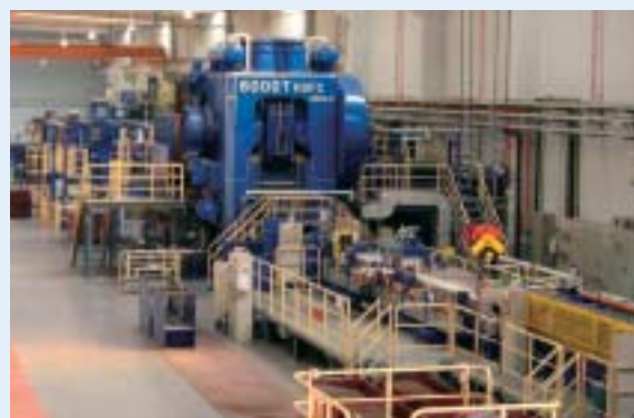
Manufacturing line for forged crankshafts used in automobiles (Huizhou Sumikin Forging Co., Ltd.)
