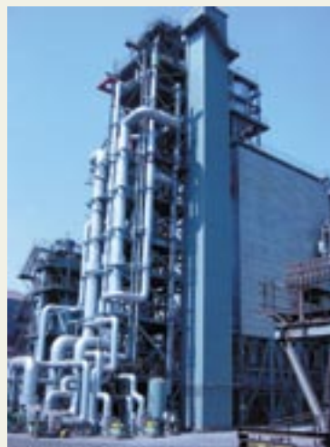
Sintering plant exhaust gas dust collector that uses activated coke (Kashima Steel Works)
