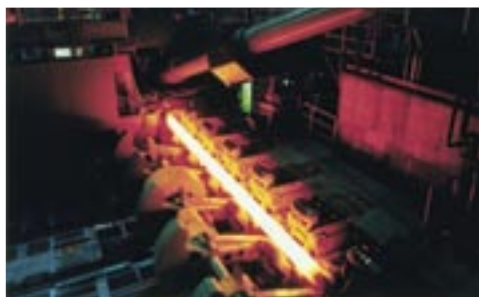
High-cross-angle cone-type piercer
