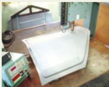
Door panel undergoing performance evaluation
