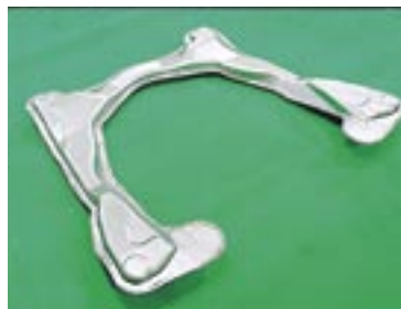
Prototype suspension member created by hydroforming
