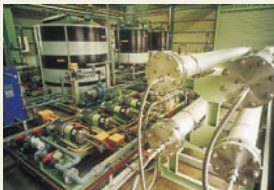
Pressure-dialysis acid recovery system (Sumitomo Metals (Naoetsu), Ltd.)
