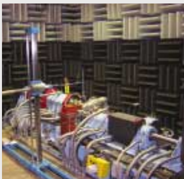
High-speed, load-applied rotation tester (in semi-anechoic chamber)
