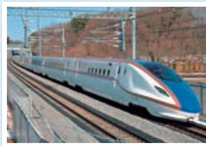
New type of railway car Hokuriku Shinkansen using the full-active suspension (Photo courtesy of East Japan Railway Company)
