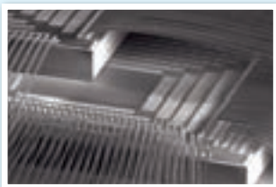
Palladium-clad new-type copper bonding wire (EX1), and example of its application
